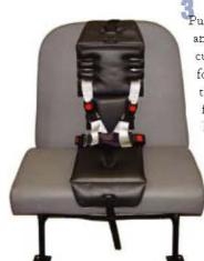
Put cushion in place and latch. Under the cushion, bring forward and connect the 1" strap to the front side push buckle (holding the pad on the seat).
