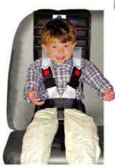
When using the Pro-Tech II Place child in seat, connect the colot coded straps together pull the ad justment straps to fit firmly across the hip and shoulder ateas.
