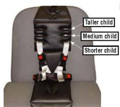
Adjust for torso heights; lower slip for shorter, middle slip for medium and upper slip for taller. Slide webbing out then into the correct slot to make the proper adjustment.
